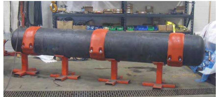
Hydrostatic pressure test set up
