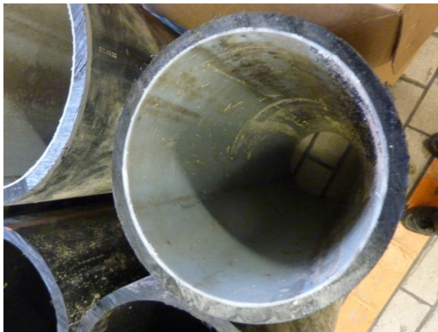
Figure 4.6 Coextruded pipes with internal layer of natural PE, Pipe G1
