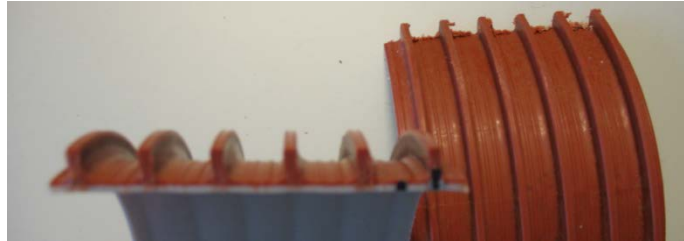
Figure 5.14 Ribs of the Structured-Wall pipe D1
