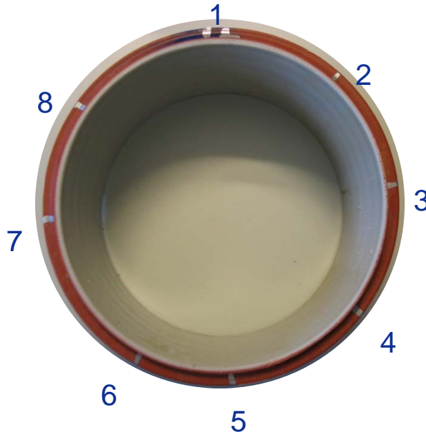
Figure 5.13 Wall thickness measurement positions for pipe D1
