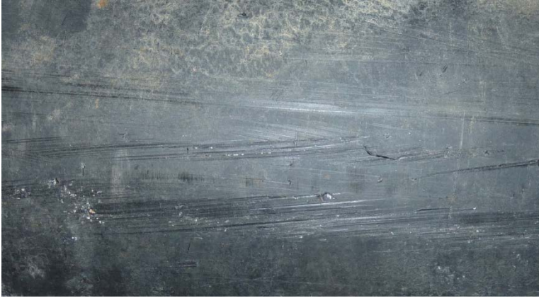
Figure 4.4 Scratches at the external surface, pipe F1
