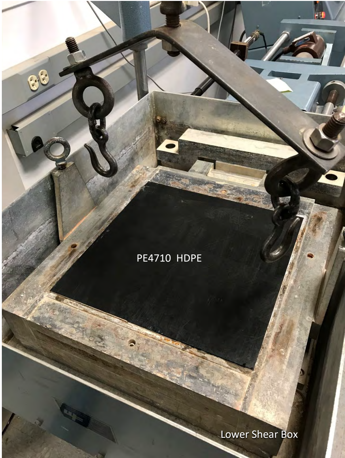
Figure 6. Image of PE4710 HDPE test coupon positioned in lower shear box.
