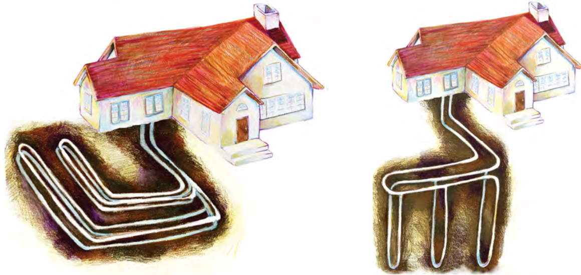
Example of a horizontal and a vertical loop geothermal installation. (Photos courtesy of IGSHPA)
