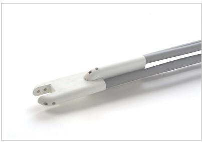
The pre-formed double U-bends are up to 335 ft in length and consist of RAUGEO PEXa pipe bent in a tight 180-degree radius and cast in a fiberglass-reinforced polyester resin eliminating the need for any fittings or joints in the borehole.
