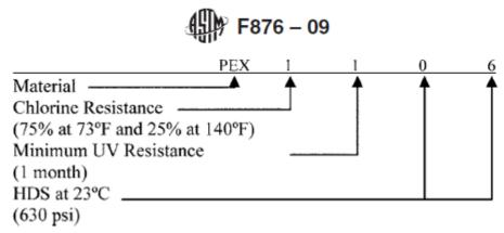
For example ASTM F876 PEX tubing marked with the material designation code PEX 1106 is a PEX tubing meeting the chlorine resistance requirement for 25% of the time at 140°F and 75% of the time at 73°F having a Minimum UV resistance of 1 month and having an HDS for water at 73°F of 630psi (HDB of 1250 psi).
