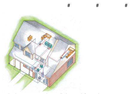
PEX plumbing systems can be installed as Trunk & Branch, Home-run, or Zoned using remote manifolds as shown in this illustration.
