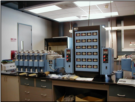
Figure IV: PENT Test Apparatus at BP Solvay Polyethylene
