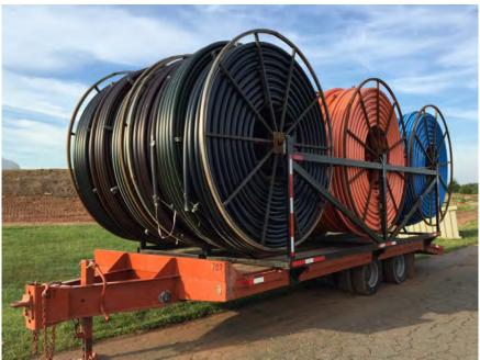
PPI's MS-5 Model Specification covers standards for HDPE conduit, which is connecting the world through expanding fiber optic networks as well as other applications.
