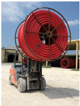
Available free on PPI's website, TN-58 "HDPE CONDUIT & DUCT HANDLING GUIDE" provides information about the safe handling of reels and coils of HDPE conduit and duct.
