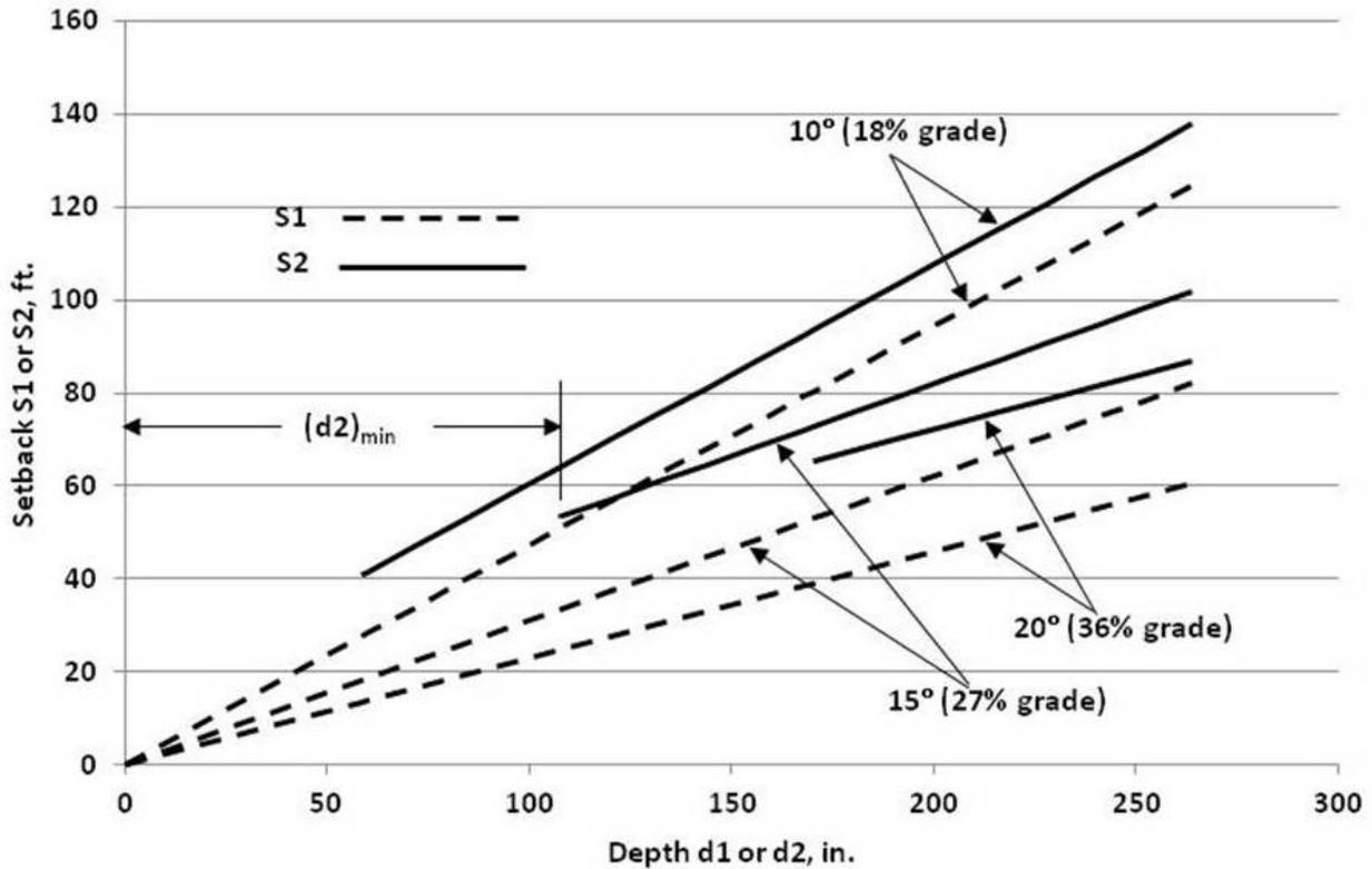
**Figure 15 Drill Rig Setback Distance**
