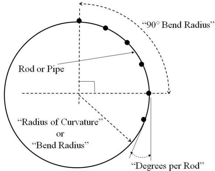
**Figure 3 Rod or Pipe Curvature Terminology**
