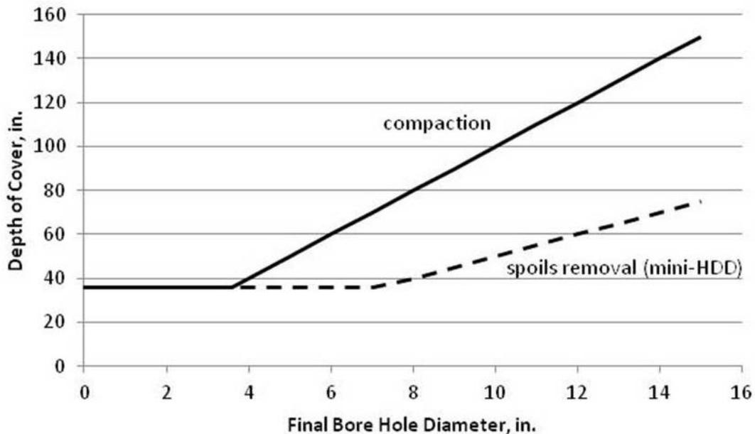
**Figure 10 Recommended Minimum Depth of Cover**
