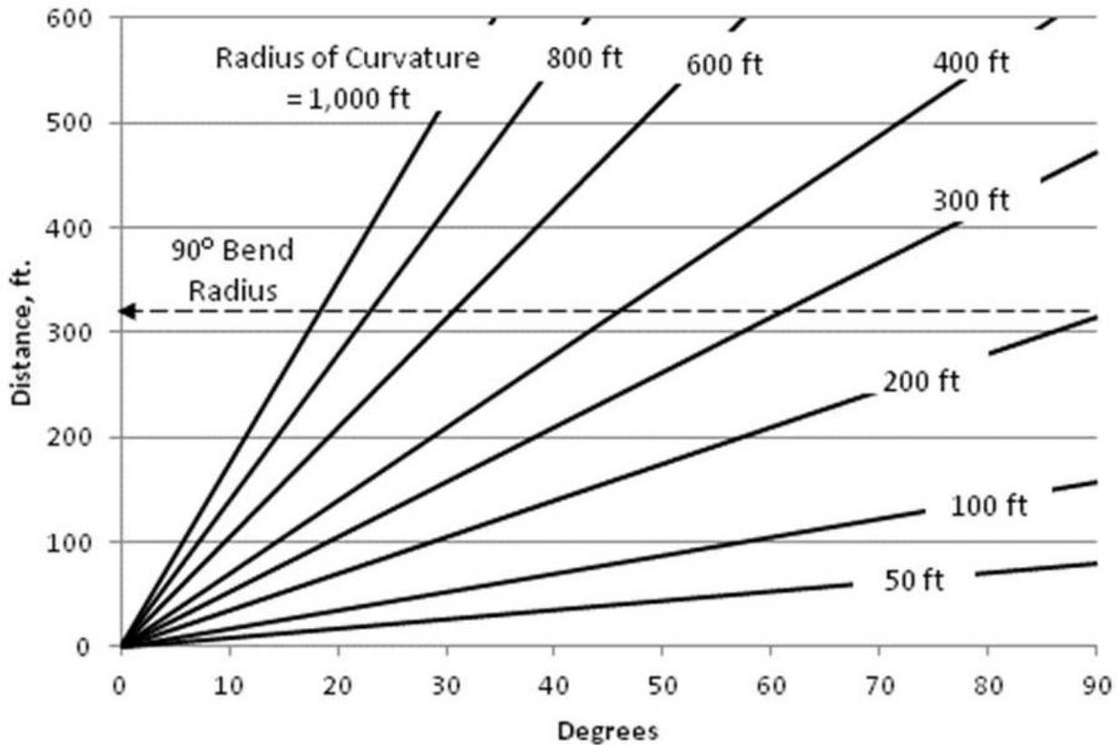
**Figure 21 Radius of Curvature for Angle and Distance**
