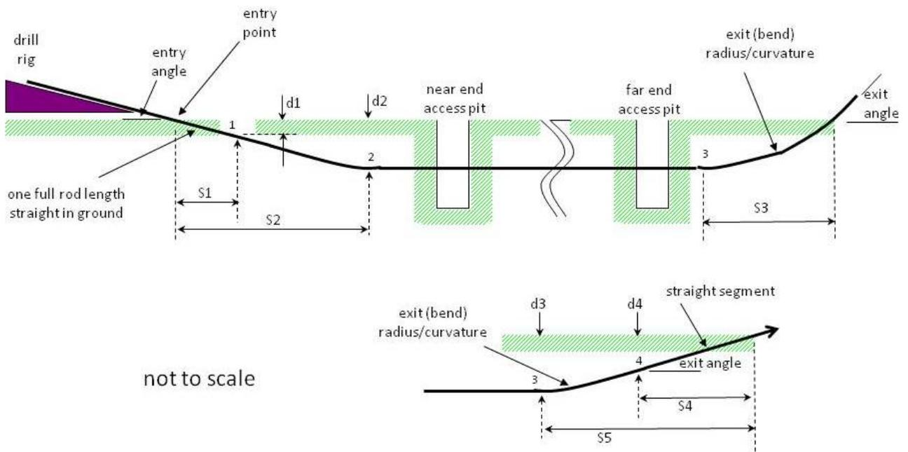
**Figure 11 Drill Rig Setup and Related Distances**
