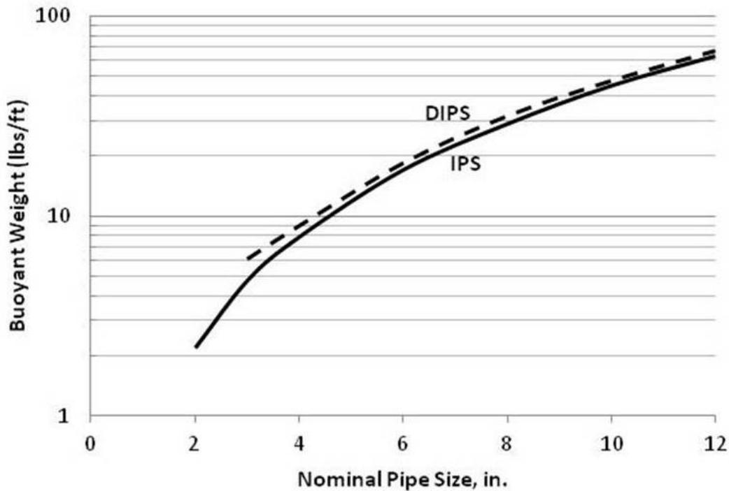
**Figure 7 Buoyant Weight of HDPE Pipe**
