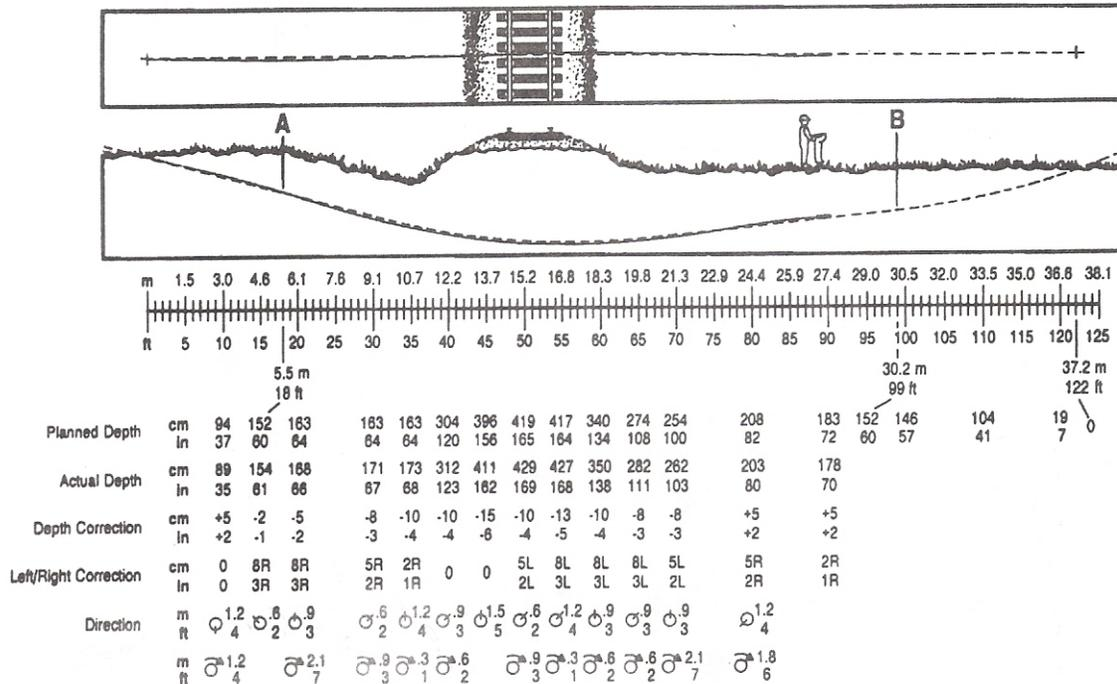
**Figure 24 Final “As-Built” Pilot Bore Path**
