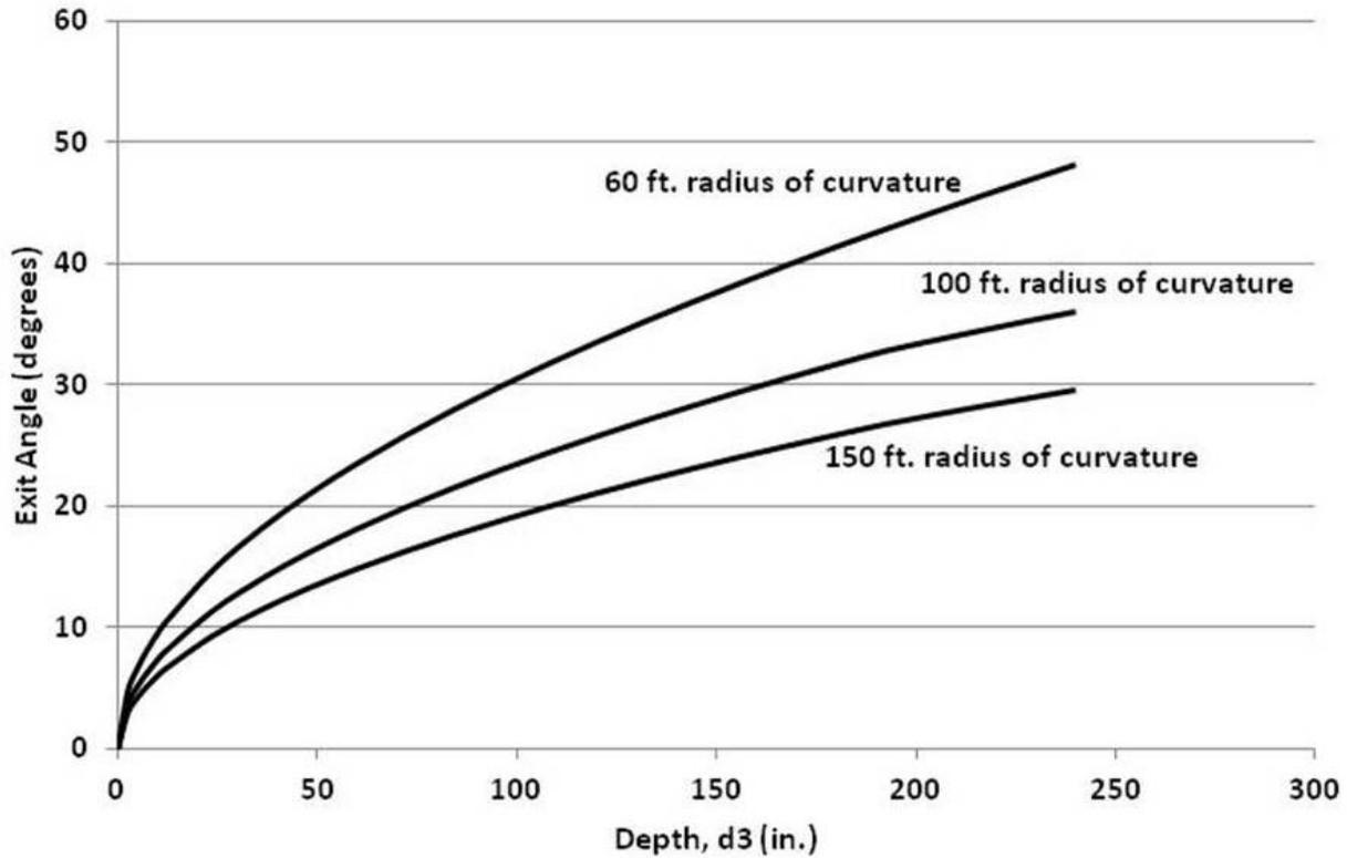
**Figure 19 Exit Angle for Rise at Constant Curvature**
