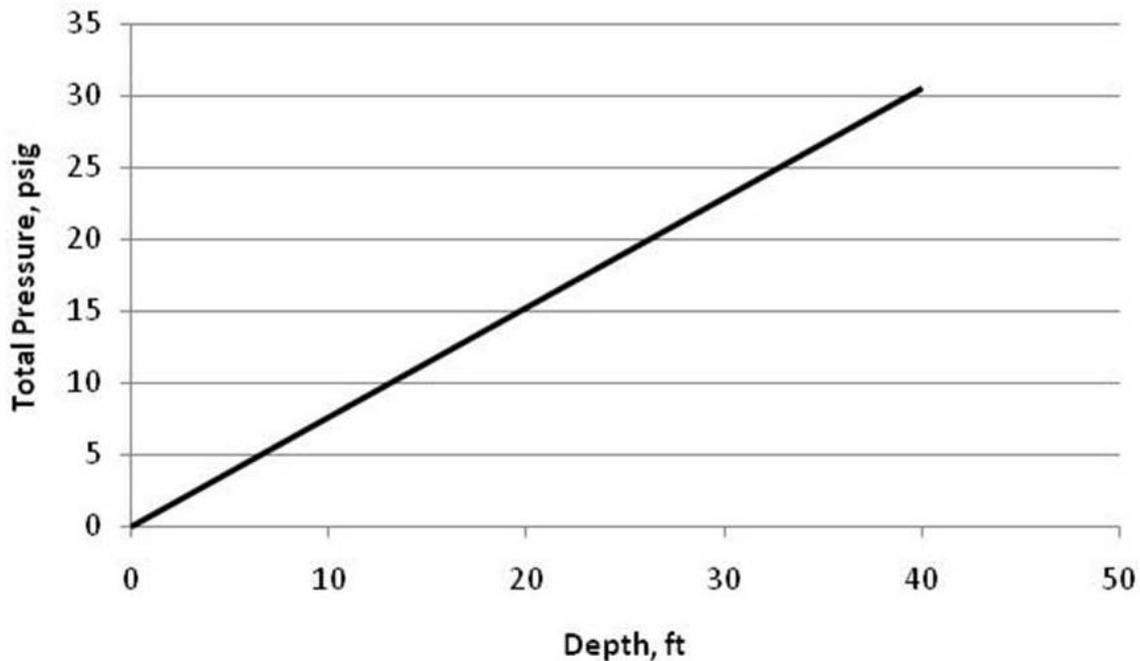
**Figure 23 Recommended Limit on Total Drilling Fluid Pressure**
