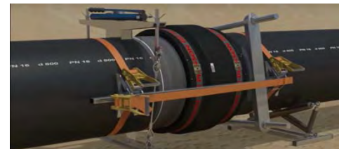
Figure III-d - Mechanical Pulling Tool
