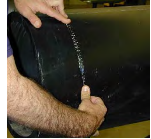
Figure IV-a - Measuring pipe diameter with Pi tape
