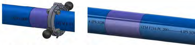
3. Scrape or peel the pipe to remove the surface layer and expose clean virgin pipe beneath.
