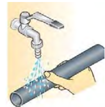
Figure X-b – Clean Pipe Ends
