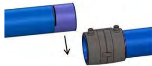
Figure X-h – Repair - Coupling Over Entire Pipe End
