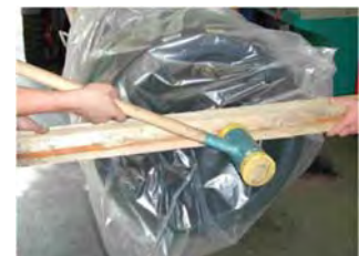
Figure X-g – Avoid Contamination During Installation
