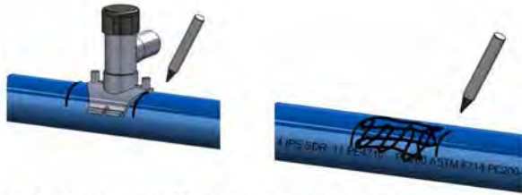
1. Mark position of saddle on pipe. 2. Mark pipe surface in area to be scraped.
