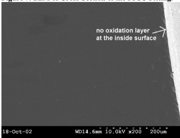
Figure 7: SEM of Cross-Section of the PPSU Fitting.
