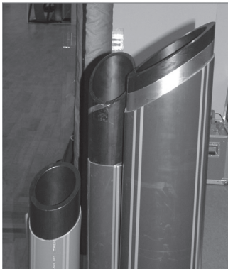
Figure 22 Protecting the PE Pipe from Shards
