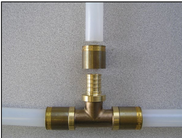
Figure 5.3 – Cold Expansion Fitting with Metal Compression Sleeve
